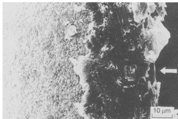
Figure 10 SEM of the fracture surface of ZTA ceramic after sinter forging at 1450 °C for 15 min and 40 MPa. A porous layer is present on the top surface (indicated by an arrow).
