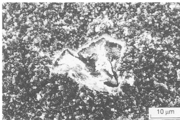
Figure 6 A cracklike defect on the fracture surface of a ZTA sample after pressureless sintering at 1500 °C for 2 h.
